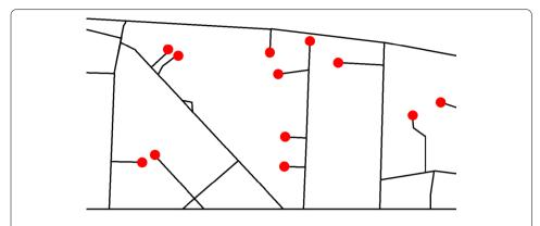
**Figure 8** Nodes with a single edge are easy to identify, and removed before computing the betweenness centrality. This example in Adur City shows how 12 nodes (red circles) can be removed, as no path goes through them
