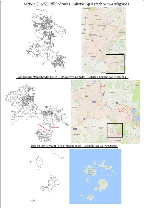
**Figure 5** Three situations leading to a largely disconnected road network. Top: hamlet for which the access clearly lies outside the main area. Middle: a very small but critical road section is administratively in another LAD. Bottom: the whole area is formed of islands
