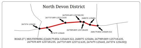
**Figure 3** Roads are encoded in a shapefile as a series of segments. A segment links two points, specified as coordinates in easting and northing coordinates. Segments are created when a road has an intersection or turns
