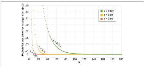
**Figure 9** Probability that the error exceeds a target (depending on  $\epsilon$ ) for different number of pivots k. Computations were performed for Cornwall
